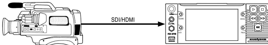
In this scenario, the video camera is the master source of the video sync. The timecode can either be read from the camera or be generated by the PIX 270i. The accuracy of the recording is dependent on the internal clock accuracy of the camera.
