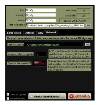
Clicking on the Network tab will present you with options to store an .xml file on the computer, that may be used to access measurements in near real time and enables the user to create any kind of custom displays either locally or via web. The .xml file will contain the majority of values created internally in 10EaZy and will enable a web-designer to access these values to create a unique display.
