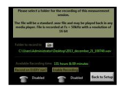
It is highly recommended to use a high capacity drive if every show is to be recorded as the recording is in uncompressed .wav format to ensure the possibility of post processing and analysis if needed. As such the risk of running out of free space on for instance the system drive is to be considered.
