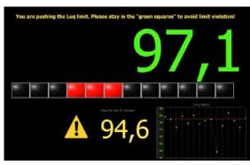
A flashing warning is triggered – Risk of limit violation if level is not reduced to a level where only green squares are lit.
