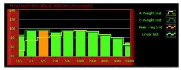
RTA limit monitoring is on – current value exceeds limit - notice that the actual limit violation is at 1 kHz, while the loudest frequency is at 125 Hz
