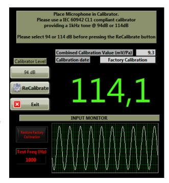
**NB:** Allow a settle time of at least 30 seconds from connecting the microphone to the sound card, before calibrating the system, to ensure that the measurement chain has reached an equilibrium state.
