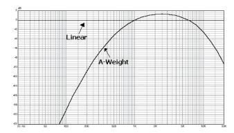
calculating the dB value. Doing so gives a more qualitative estimation of the "danger" posed to the ear for a different sound level. If an electric bass is measured with and without the A-weighting, the dB value will be very different, because the A-weight filter attenuates the low frequencies.
