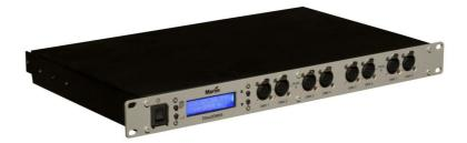
Ether2DMX8 is a highly capable DMX router and much more! As a DMX router, it translates Art-Net protocol into DMX in/out universes but can also be used as a DMX merger, DMX splitter hub, fail safe device, cue playback, and DMX viewer monitor. As an extension for the M1 and M2GO console it provides 8 additional DMX ports and includes the required DMX license. When connected to a standalone PC, the Ether2DMX8 also becomes the license key for M-PC and provides 8 DMX Universes.
