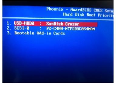
Arrow Down to the USB Drive (e.g. SanDisk) and use the + key on the keyboard until the USB Drive is on the top of the list.
