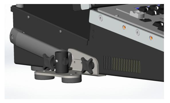
Place the Magic Arm into the back of the screen mount and tighten the thumbscrew to it fits the ridge in the pin of the arm. Then place the screen and arm into the mounting hole on the console bracket.
