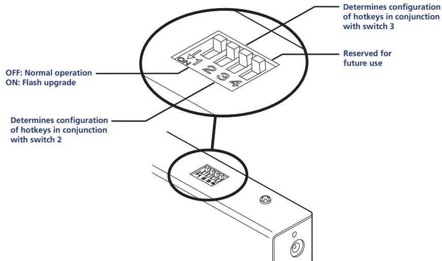
*Note: When shipped, all switches are set in the OFF positions and this will produce normal operation.*
