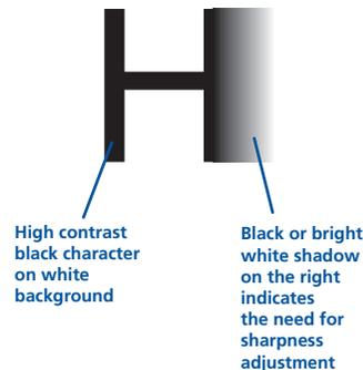
*Note: The Word processor method is accurate and quick. However, for the very finest video compensation, use the latest Adder "skew" test pattern program which shows both the skew pattern and a section of mixed size Hs (black on white and white on black).*
