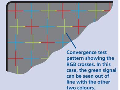
The screen will show a series of fine red, green and blue crosses which should all be in line, vertically and horizontally. Skew affects the horizontal placement of the colours and using this pattern it is much easier to discover which, if any, colours are being adversely affected by the cable link.
