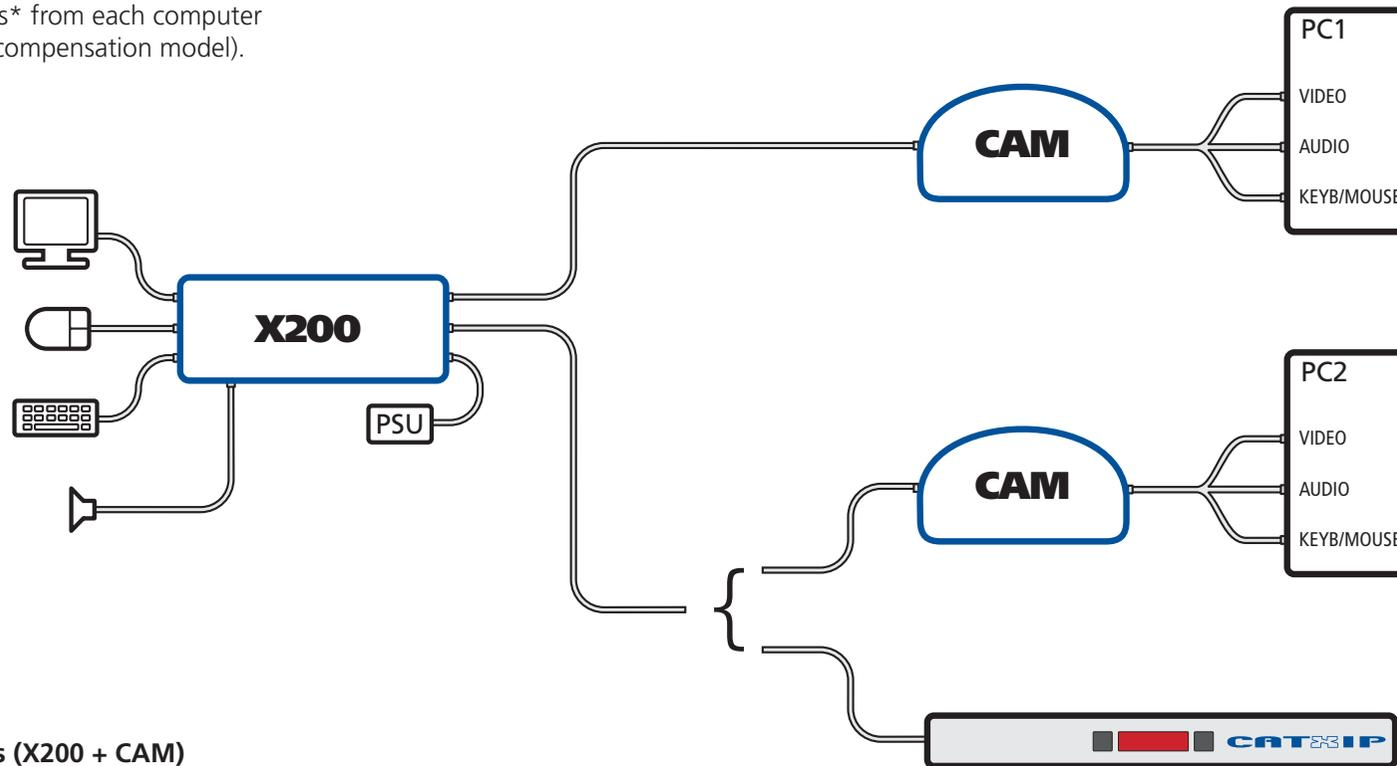
X200 modules can be used to connect to individual computer systems via CAMs or to many computers via AdderView CATx switches
