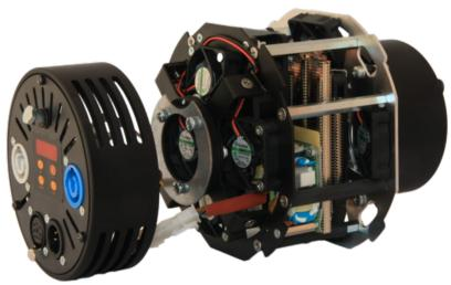
The HPLed is powered by an high power Light Emitting Diode Array with a standard Colour temperature of 3200°K and 5600°K. HPLed incorporates a display board to operate the fixture via RDM and or DMX Protocols. The rear section of the RDM/DMX HPLed embeds functions to facilitate fixture operations, such as convenient IN/OUT 5-pin XLR and PowerCon connectors.
